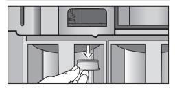
Pull the rubber connector downwards.
